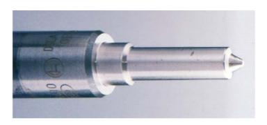
This is a fuel-injection nozzle. The exit nozzle is a hole only 50 microns in diameter and 1 millimetre in length and strict requirements on the roughness of the sidewalls. This can only be achieved by the lasers machining with exceptionally high beam quality. The results are impressive: There is a 25% reduction in soot particle emission, and a 35% reduction in unwanted hydrocarbon emission.
